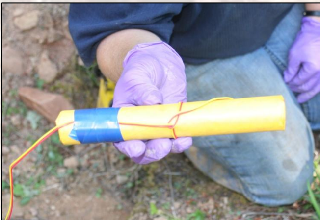
One half pound stick of dynamite with blasting cap
