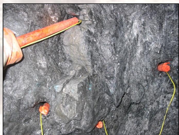
(left) A student and I run a pneumatic drill at an Oregon gold mine. (above) One-pound dynamite sticks loaded into boreholes cutting a tunnel in a Colorado gold mine.
