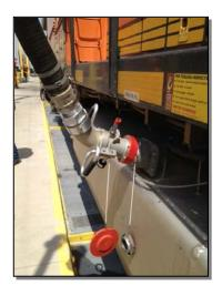
The fueling platform was then tested using the SpillX components installed on locomotive 4715 and a nozzle installed on crane 1 of the platform. Approximately 1,250 gallons were added to the tank at a rate of 534 gpm.
