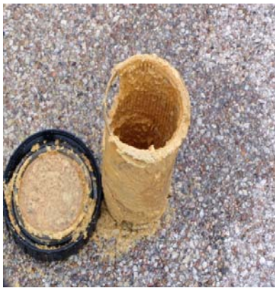
Inorganic Fouling of Screen and Bag Filters
