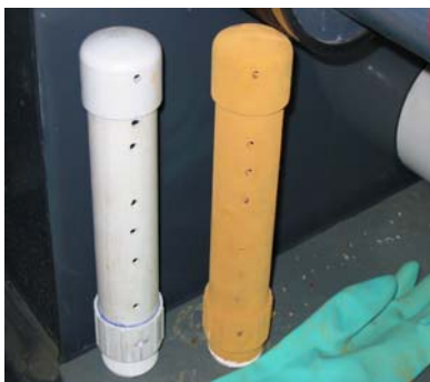
Inorganic Fouling (Iron) of Air Sparger
