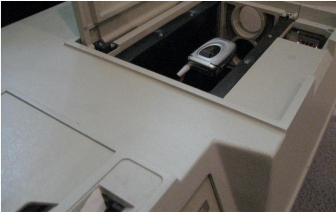
**Figure 3:** To measure rewinding, an aqueous sample of human DNA is placed in a cuvette inside a Hewlett Packard spectrophotometer which measures the absorption of UV light by the sample. Light absorption is measured every 10 seconds when the DNA is spontaneously rewinding. Note the position of the cellular phone whose radiated EM field influences the rewinding process of the DNA inside the cuvette underneath the cellular phone.
