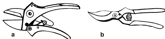
Figure 1. Hand shears. (a) anvil type, (b) scissors type.
