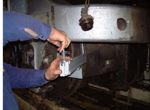
Fig. 6 Insert lock pin, and check all fasteners to ensure they are tight. Make sure to check stick adjustment to the wheel. Stick should be adjusted into the throat of the flange. See fig 4 above.
