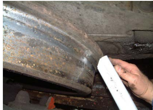
Fig. 4 Ensure magazine alignment to wheel is \frac{3}{4} " clearance, with outside edge of magazine slightly below top of flange. Stick will be centered in throat of flange. Some stick on tread of wheel is OK.
