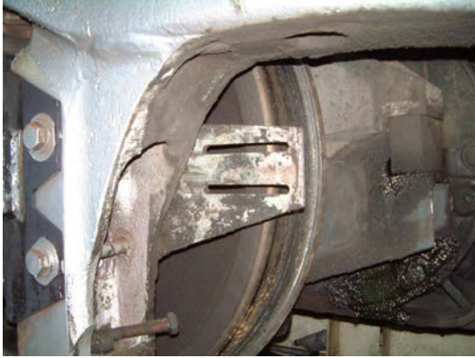
Fig. 1 Remove spray nozzle, bracket and hoses if equipped. Pedestal bracket as shown from spray system may be re-used for the stick system. NOTE: MPL pedestal liner mounting bracket supplied with each set, mount to ped liner as shown.
