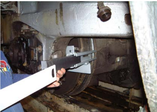
Fig. 5 Insert lube stick as shown. Ensure spring is on spring slide and insert slide / spring assembly into the guide slots on the magazine. Hold spring slide in until pin is inserted in magazine holes.
