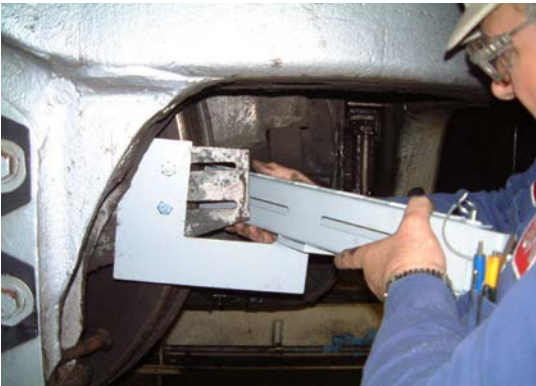
Fig. 3 Magazine assembly may be mounted either side of bracket depending on distance from wheel. If there is room to use four magazine bolts do so, or secure with two bolts, nuts, washers.
