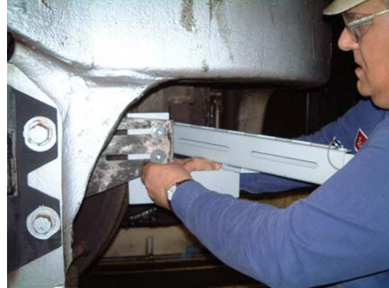
Fig. 2 Mount magazine assembly to bracket as shown. Set brakes to move wheel toward end of magazine to Ensure \frac{3}{4} " clearance to wheel.
