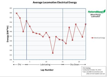
Once it was determined that the train had established a steady state friction reduction based on the energy measurements the train was stopped and the flange lubrication sticks were removed. The sticks were then measured to determine wear rates over the 35 miles traveled during testing.
