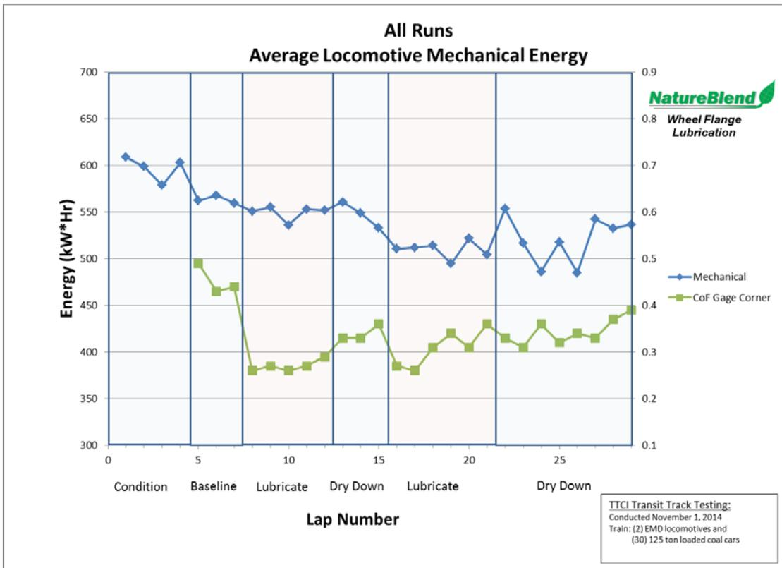
Of note in the charts above is NatureBlend’s ability to immediately reduce the gage face CoF with each application of the product. Due to the limited time available for testing, we were not able to return the track to the original 0.44 CoF; however the chart demonstrates with a reduced gage face CoF, the energy measurements were consistently lower than with a dry rail.
