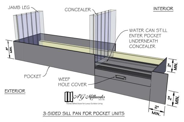
NEED TO HAVE 3-SIDED SILL PAN WITH WELDED CORNERS FOR THE POCKET. THIS WILL PREVENT WATER FROM PENETRATING INTERIOR.
