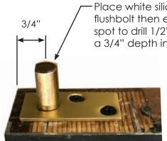
Place white silicone on tip of flushbolt then engage to mark spot to drill 1/2" diamter hole at a 3/4" depth into the head jamb.
