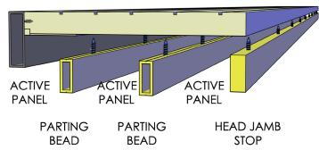
INSTALLATION OF INTERMEDIATE PANELS: (From the Interior) Place the wheels of intermediate panels on the track behind pocket panel and tilt the top of the panel upward into position. Be sure that the stiles overlap so that the check rails on the two panels will connect and form a seal. Check to be sure the panel rolls properly.
