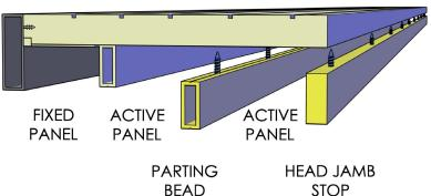
**INSTALLATION OF INTERMEDIATE PANELS: (From the Interior)** Place the wheels of intermediate panels on the track behind fixed panel and tilt the top of the panel upward into position. Be sure that the stiles overlap so that the check rails on the two panels will connect and form a seal. Check to be sure the panel rolls properly.
