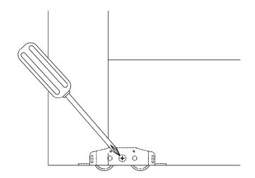
The weight of the panel may interfere with the adjusting mechanism. Before adjusting have helpers lift the panel up either by hand or with the aid of suction cups on the glass to alleviate the pressure on the wheels .
