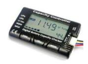
Figure 23: Battery tester
