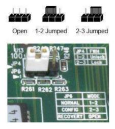
Figure 31: Jumper Setting
