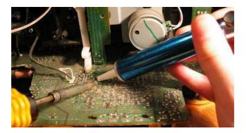
Figure 28: Desoldering
