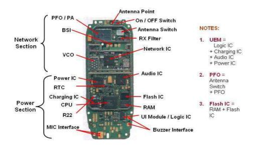
Figure 5: Parts of a mobile phone
