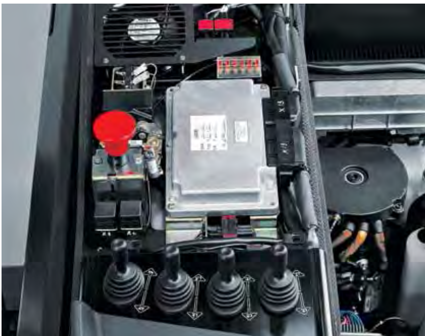
Efficient conversion of energy to motion. Linde Digital Control with CAN bus connection.
