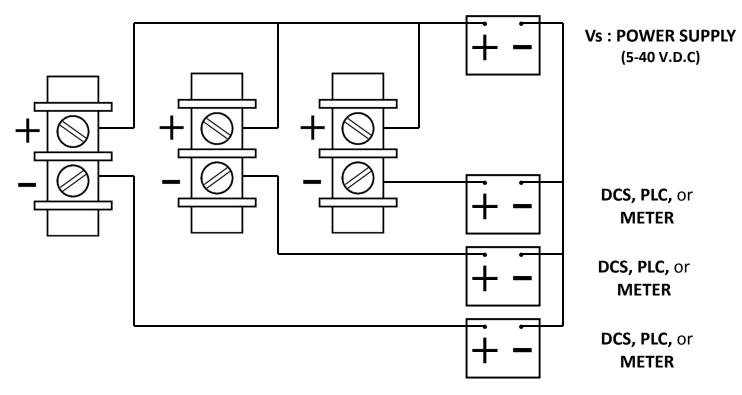
Power Supply should be rated for a current of no less than 25m.A. x no. of sensors in Loop.
