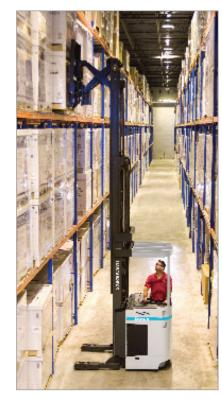
SRX offers advanced anti-rollback protection, ideal for minimizing push-back when placing loads.
