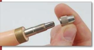
**Step 2**Remove the chuck shaft from inside the pin vise.
